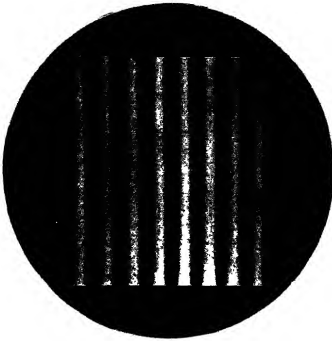
FIG. 132.—Black Central Band and equidistant Spectrum Bands on each side, afforded by Babinet's Composite Plate of two Quartz Wedges, one parallel and the other perpendicular to the Axis. (Direct Photograph of Screen Picture as projected by Lantern Polariscope)
